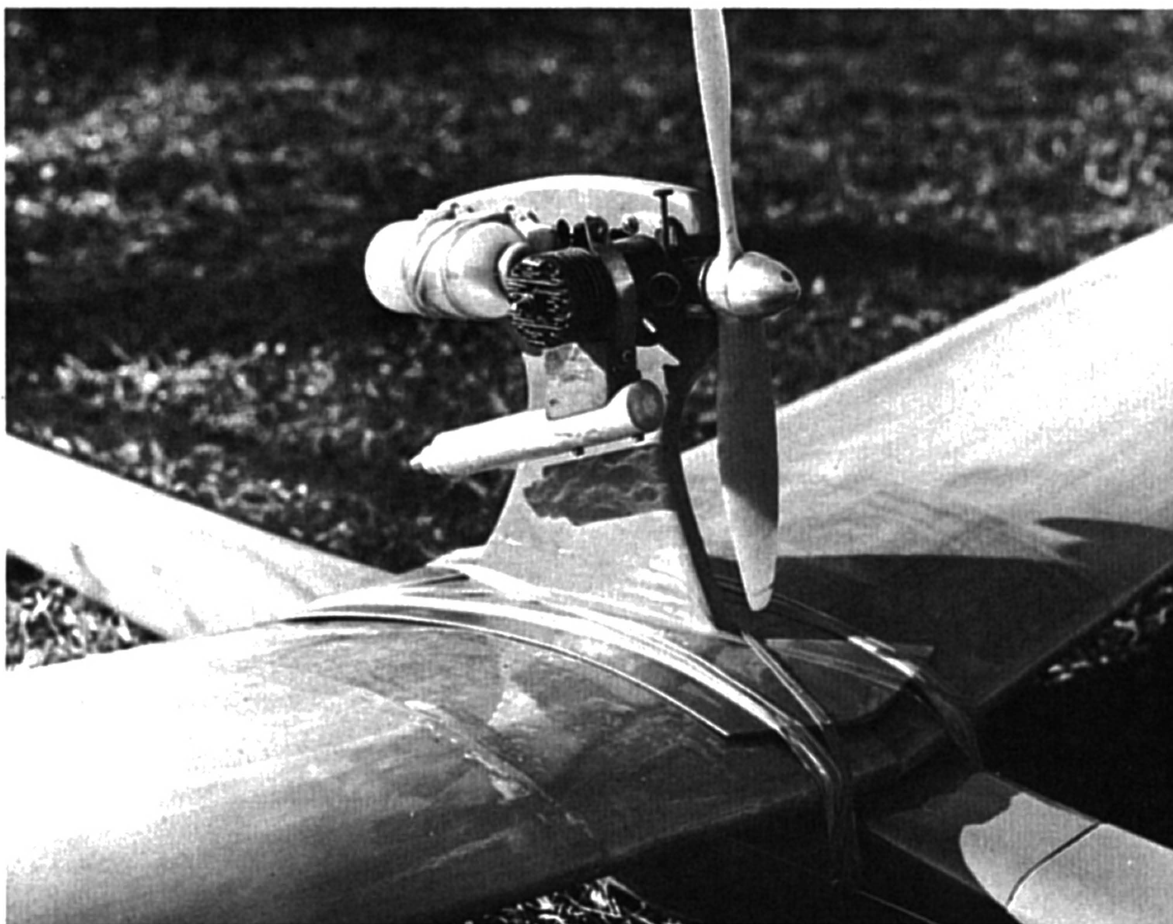
Large engine and small tank work as well as large tank and small engine, but author recommends the fast climb on powerful but light Fox 35 engine. Power pod could be streamlined considerably; it noticeably hinders the glide of King Kong.
